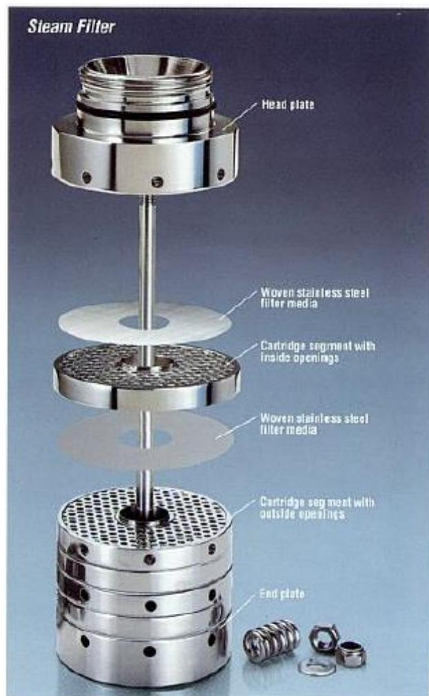
The patented segmented construction of MICROPURE filters offers significant advantages over conventional cartridge filters (shown above). Steam flows into the openings on the outside of each segment disc and passes through the filter and into an adjacent disc. Filtered steam exits through the opening at the center of the cartridge, free from contaminants that can affect the quality of your product.
