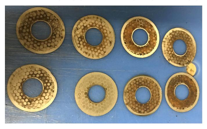
Picture showing impurities removed from steam flow on stainless steel media.
