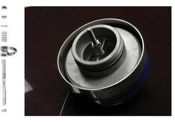
Unit is compressed and held together with compression spring.
